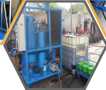
VACUUM SYSTEM (DEHYDRATION)
